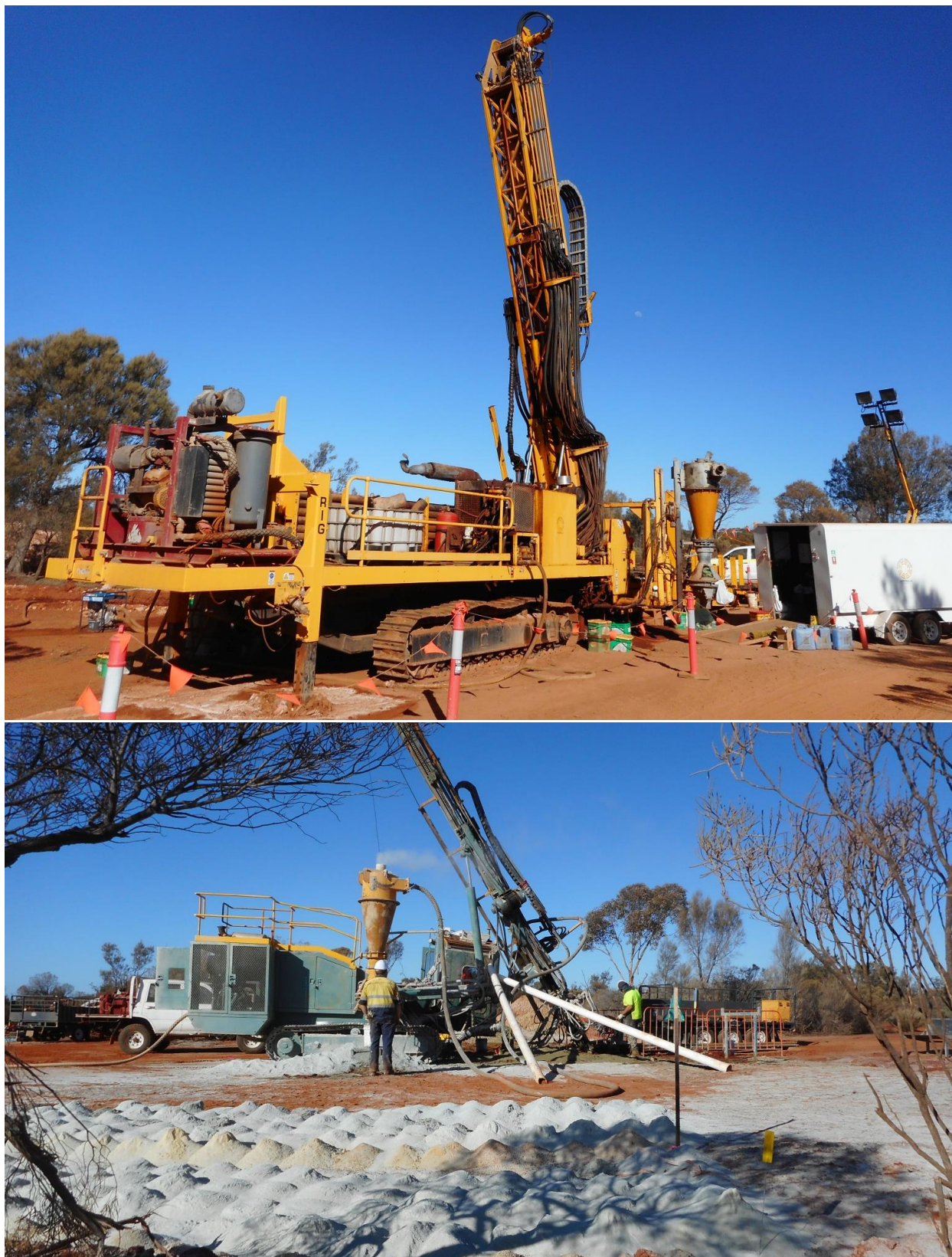
Figure 4: Top – Hydco RC / DD Rig provided by Topdrive Drillers during the coring of CBDD053. Bottom - RC / Diamond Rig provided by DDSR Australia drilling a series of precollars prior to diamond tails.
